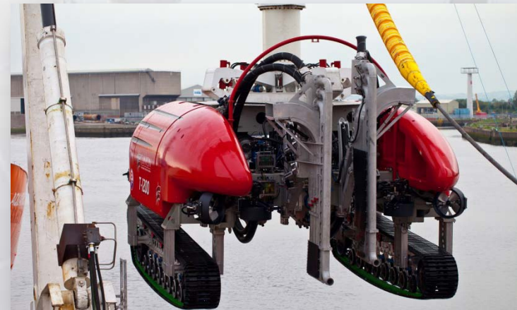
T1200 Jet Trencher preparing for deployment
