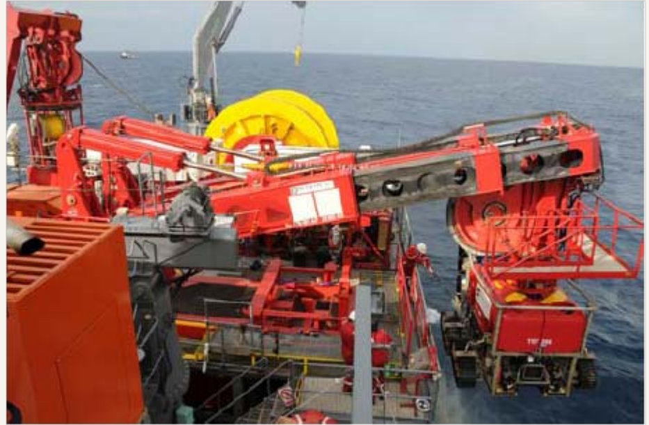
Cable trencher T200 being launched from the Seacor Canyon offshore Indonesia
