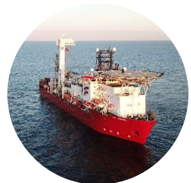
Well Enhancer (North Sea) DP3 light well intervention and saturation diving vessel
