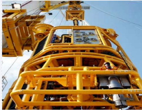
Intervention Riser Systems
