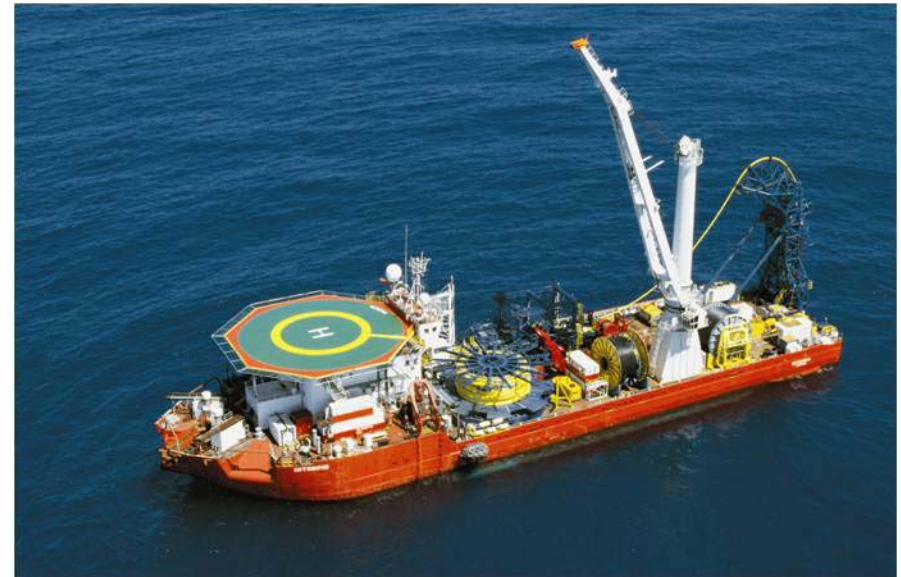
DP Reel Lay Vessel Intrepid
