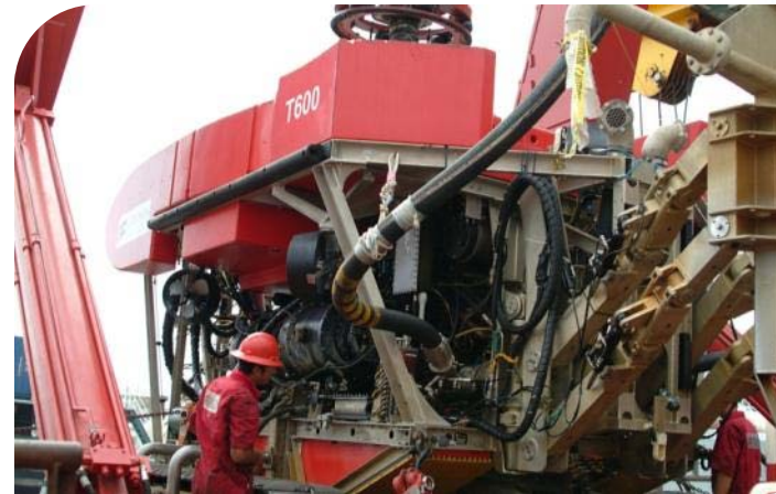
Trenching ROV preparing for deployment
