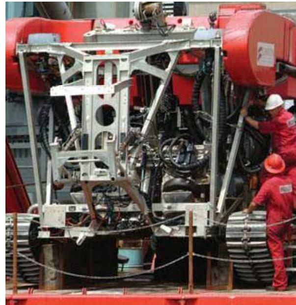
The 600 hp Supertrencher II system is designed to operate at water depths in excess of 6,500 feet.
