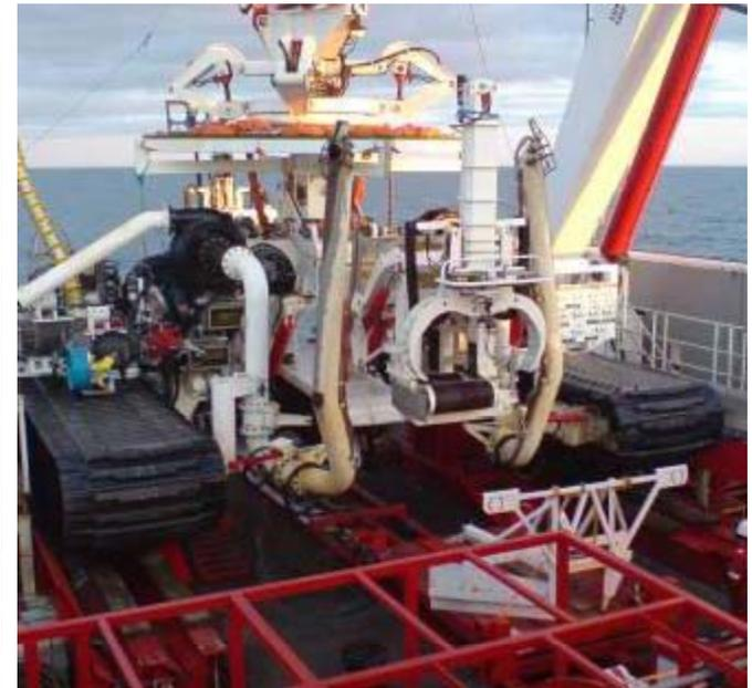
The state of the art I-Trencher system trenches, lays pipe up to 16" in diameter, and backfills in a single operation.
