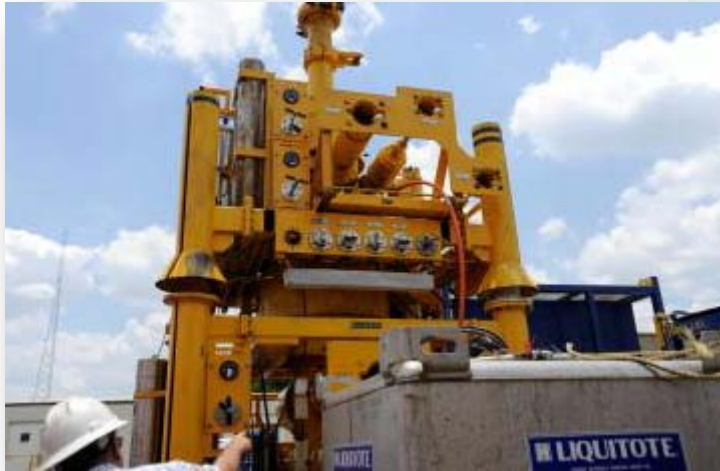
Intervention Riser System
