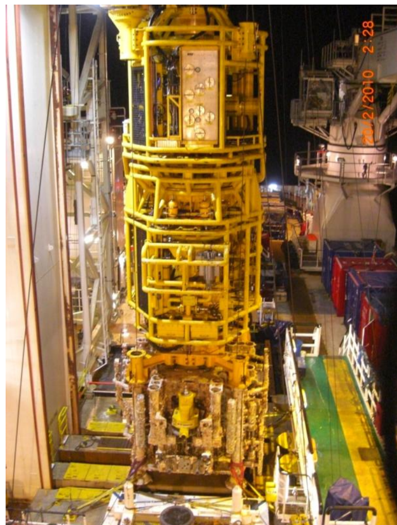
Wellhead, tree and SIL lower intervention package recovered by the MPT on the Well Enhancer
