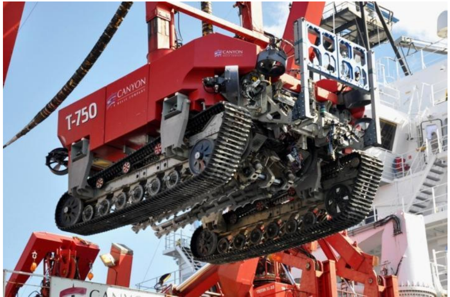
T750 trencher being launched from the deck of the Island Pioneer
