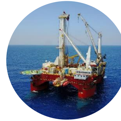
Q4000 (Gulf of America/ West Africa) Dynamically positioned class 3 (“DP3”) purpose-built semisubmersible well intervention vessel
