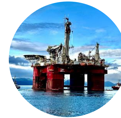
Q7000 (West Africa / Asia Pacific / Brazil) DP3 purpose-built semisubmersible well intervention vessel
