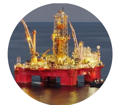
Q5000 (Gulf of America) DP3 purpose-built semisubmersible well intervention vessel
