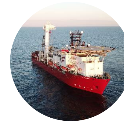
Well Enhancer (North Sea) DP3 light well intervention and saturation diving vessel
