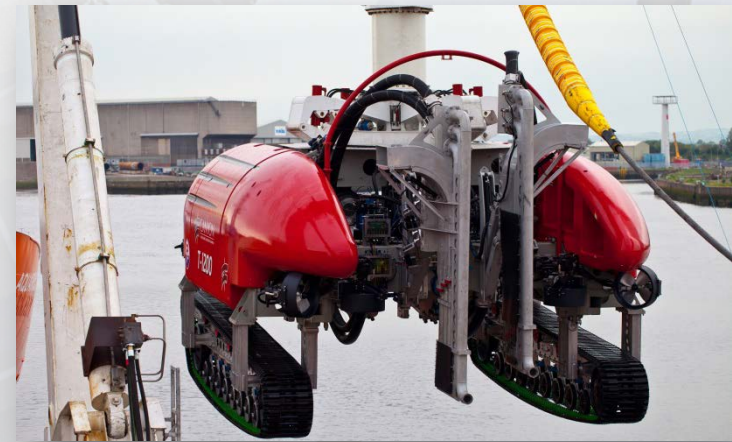
T1200 Jet Trencher preparing for deployment
