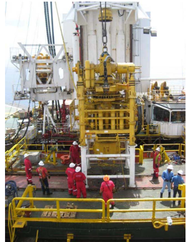
Q4000 Intervention Riser System in operation
