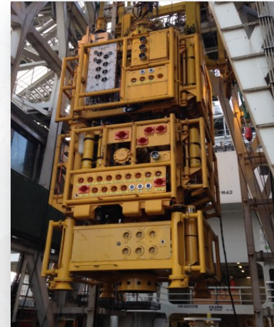
Intervention Riser System
