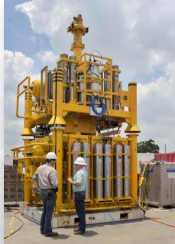
Intervention riser system undergoing testing
