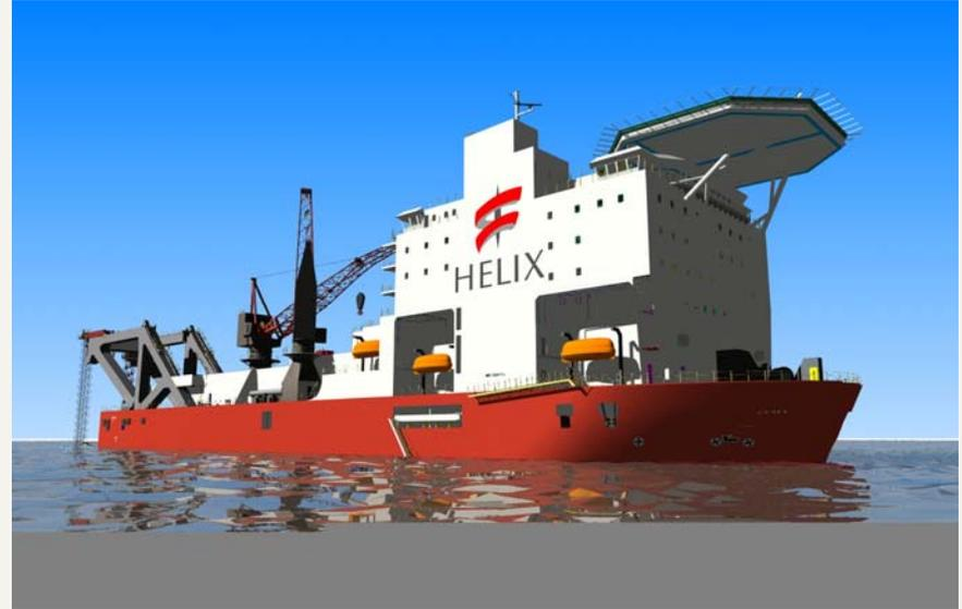
***Caesar is among the world's largest deepwater construction vessels, a "floating factory" capable of laying pipelines up to 42 inches in diameter***
