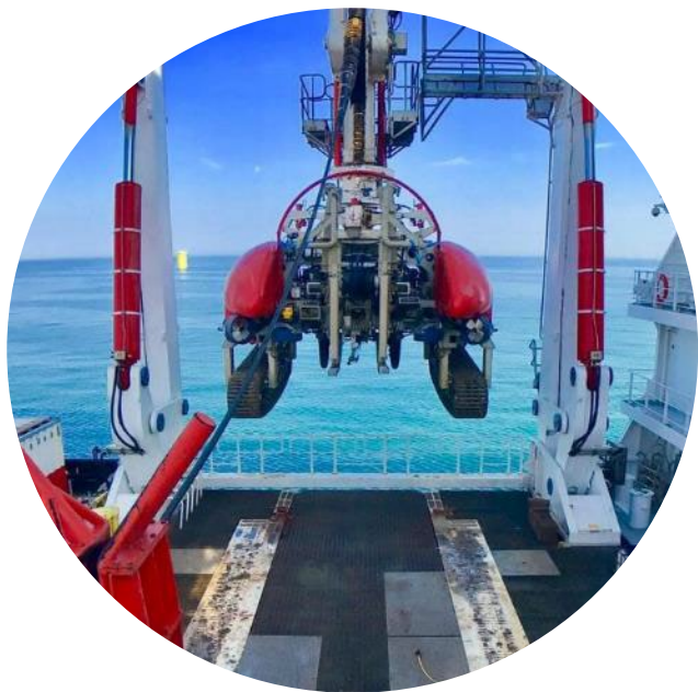
Subsea Trenchers (6 units)
