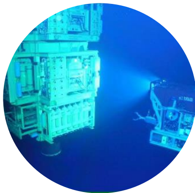
Intervention Riser Systems Utilized for wireline intervention, production logging, coiled-tubing operations, well stimulation and full P&A operations
