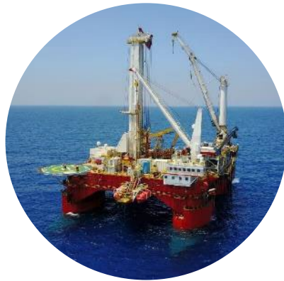
Q4000 (Gulf of America) Dynamically positioned class 3 ("DP3") purpose-built semisubmersible well intervention vessel
