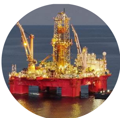
Q5000 (Gulf of America) DP3 purpose-built semisubmersible well intervention vessel
