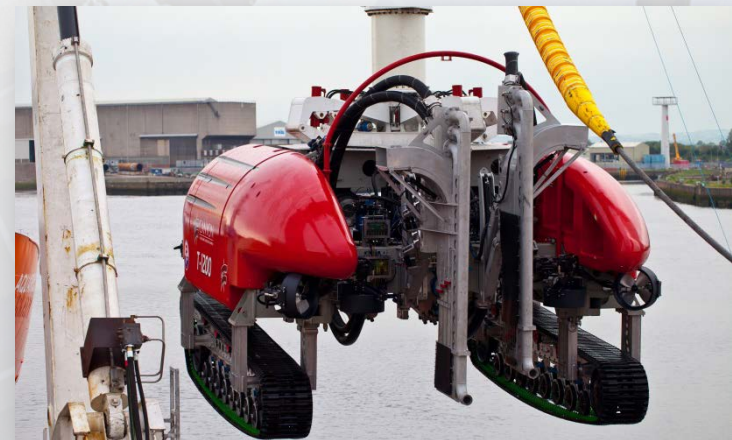
T1200 Jet Trencher preparing for deployment
