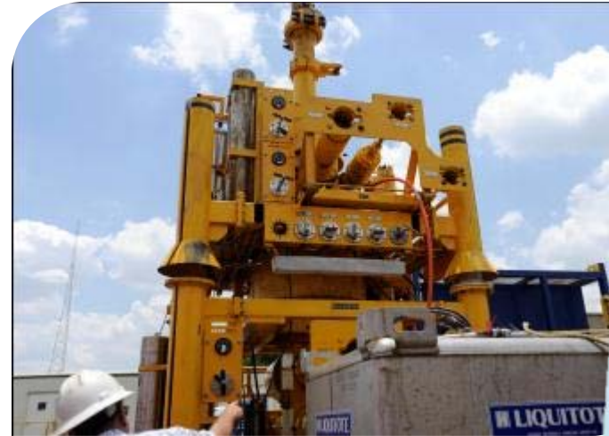
Intervention Riser System
