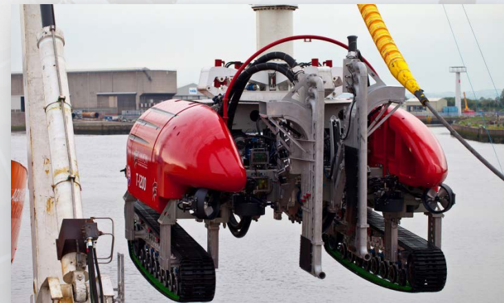
T1200 Jet Trencher preparing for deployment
