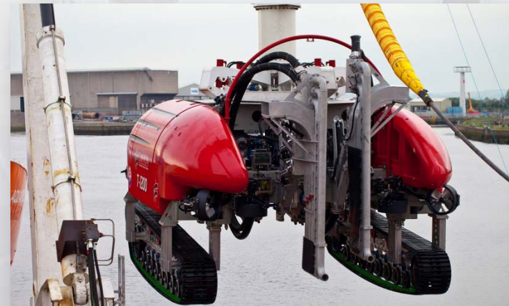
T-1200 Jet Trencher preparing for deployment
