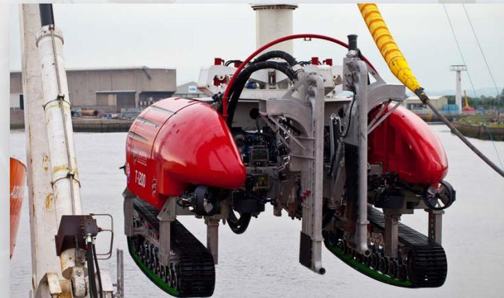
T1200 Jet Trencher preparing for deployment
