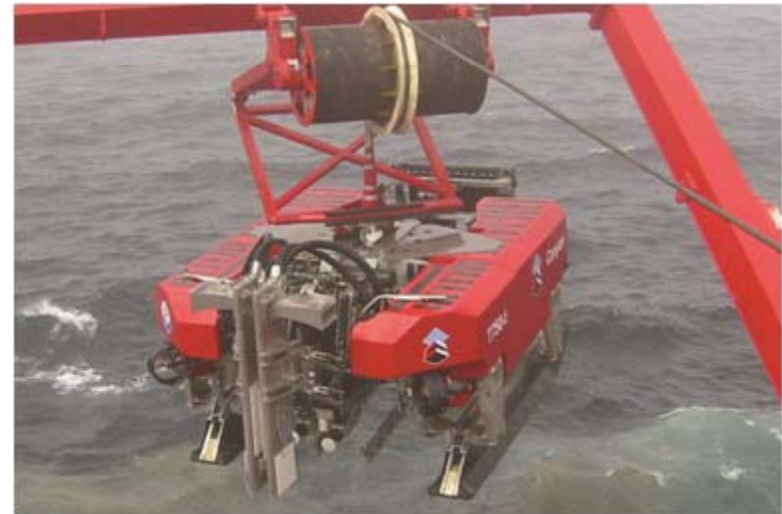
T-750 being deployed for trenching work in the North Sea
