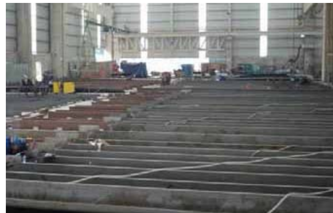
Various components of the Grand Canyon's hull being fabricated and welded in Turkey
