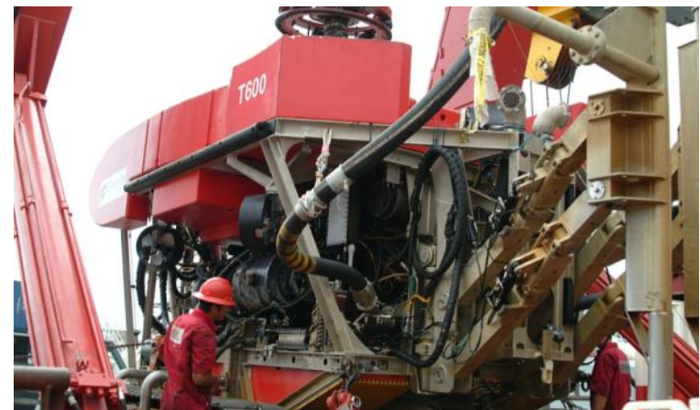
Trenching ROV preparing for deployment
