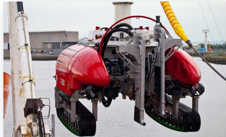
T-1200 Jet Trencher preparing for deployment
