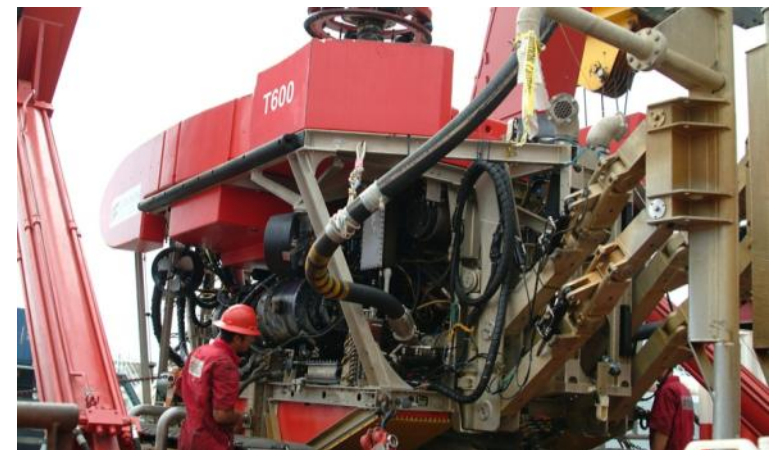
Trenching ROV preparing for deployment
